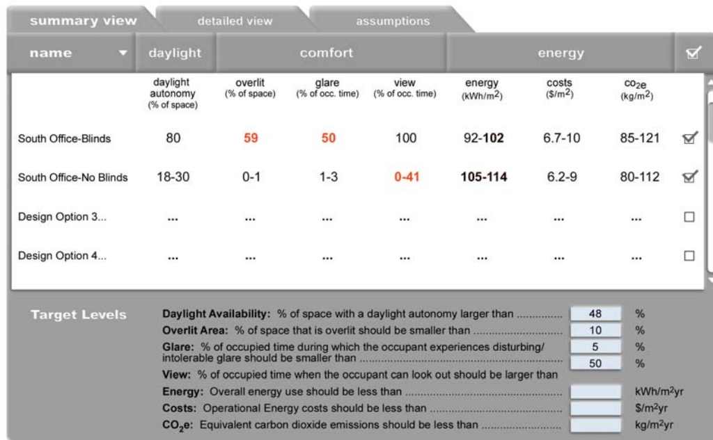
Figure 14: Daylighting Dashboard (summary view).
