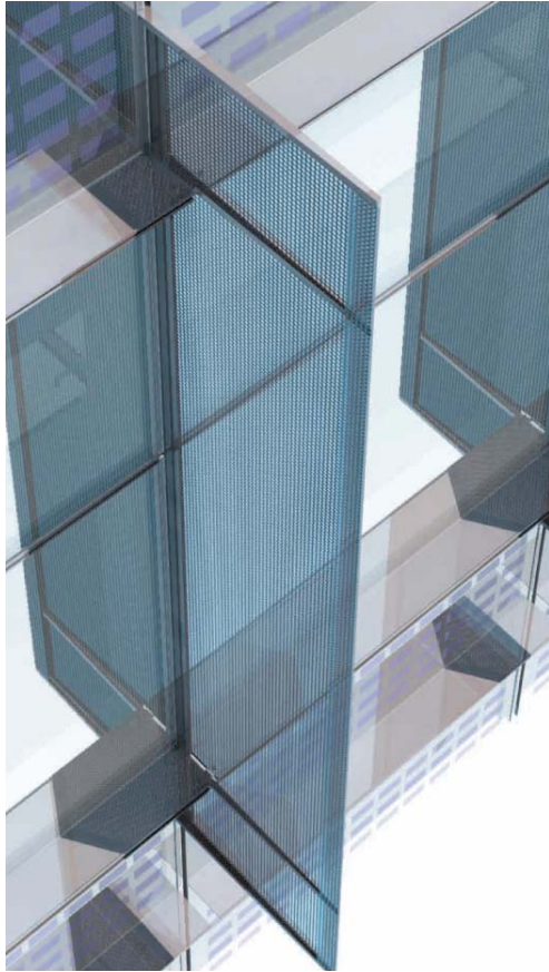
Left: Vertical fin, perforated design
