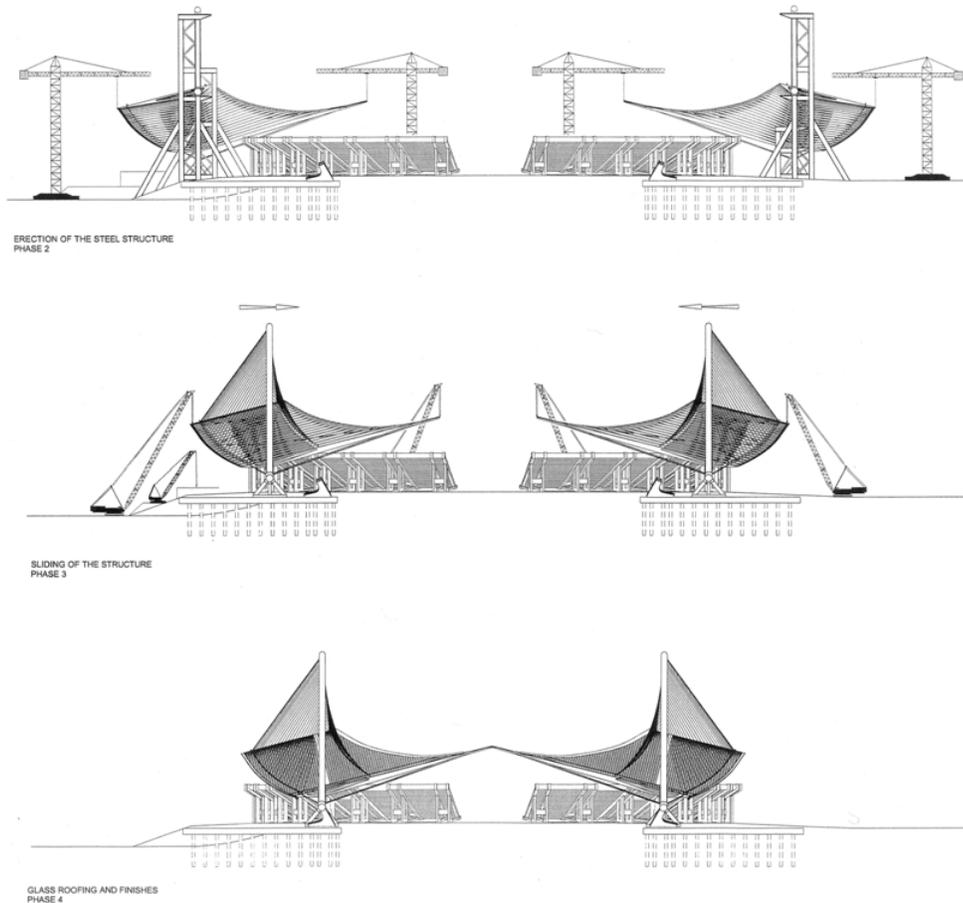
**Fig. 16.** The construction and sliding phases.
