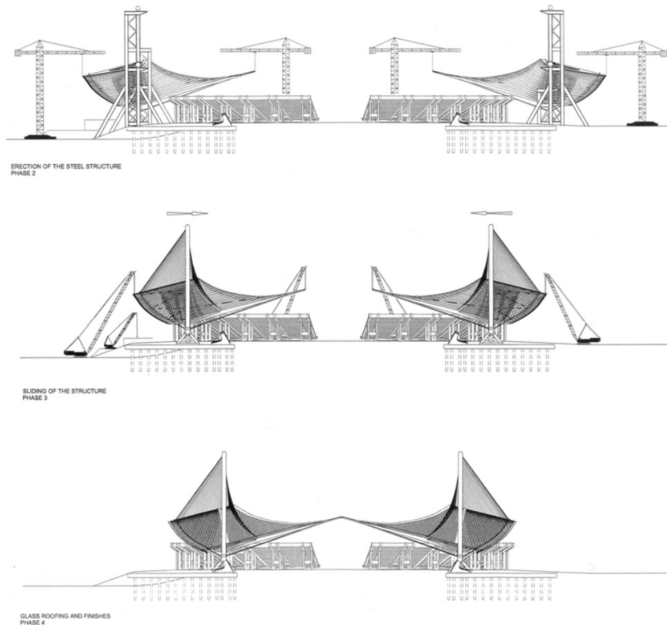
**Fig. 16.** The construction and sliding phases.
