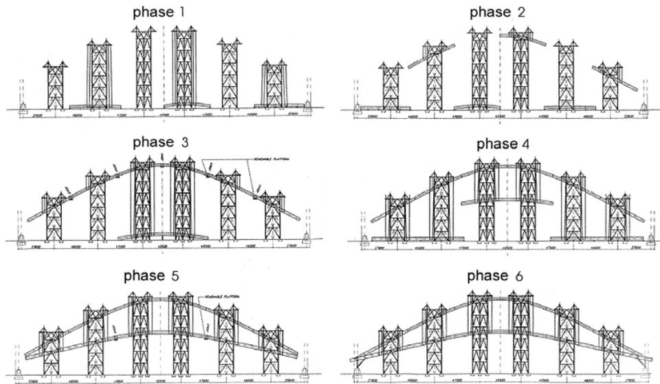
Fig. 11. The erection phases of the arches on the supporting steel towers.
