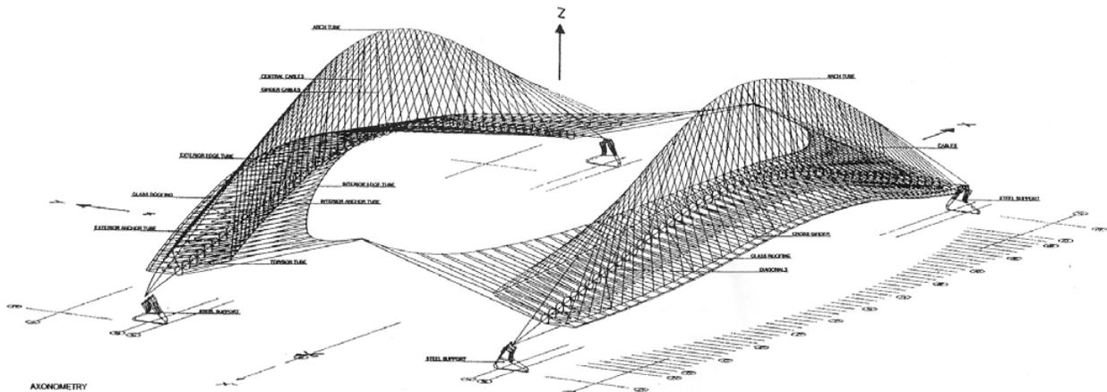
**Fig. 8.** Axonometric of the structure for the covering of the Olympic Stadium.
