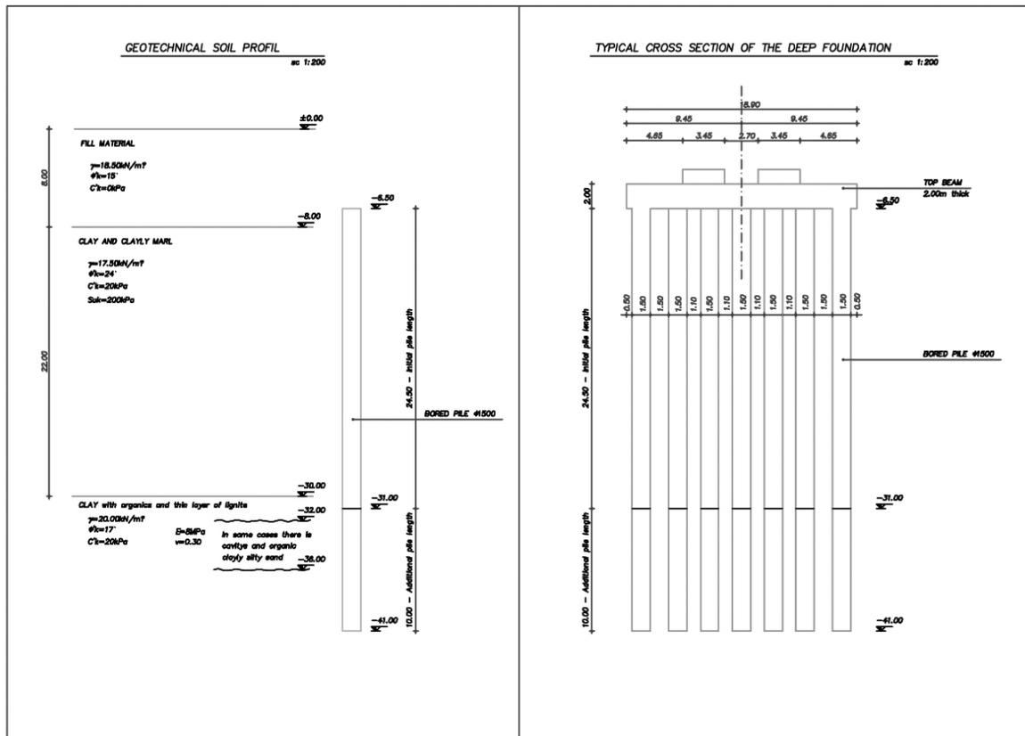
Fig.9. Diagram of the foundation method and the soil issues.
