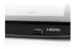
Micro HDMI: Even smaller version of HDMI usually found on smartphones and tablets. Use the Micro HDMI to HDMI adapter.
