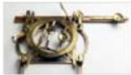
1817 John Farcy ellipsograph, a parametric drawing tool for complex curves 1817
